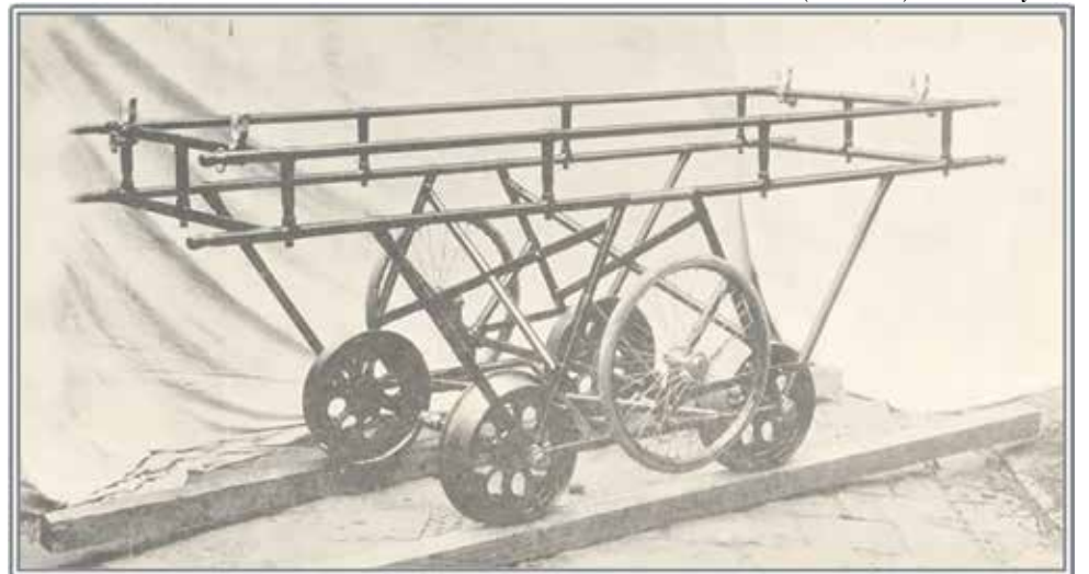
An ambulance possibly similar to the one that carried Jack Hall to the hospital. This particular one was designed to run on rails using the four steel wheels, as well as on roads using the rubber wheels in the middle. (Tasmanian Weekly Courier, 14 January 1909.)
